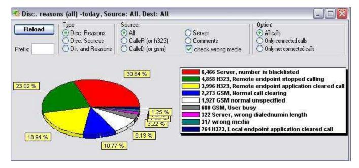
The server will collect the reason in the most appropriate format depending on the protocols used. For example for a call from voip to gsm if the disconnect was caused by the gsm party, then you will see the GSM network reason code here. Otherwise, if the disconnect source was the caller party, and then you will see H323 or SIP reason codes here.
