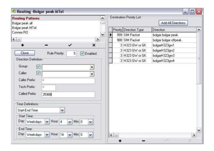
\*Tip: you don't need to enforce traffic sender rights by routing. The routing can be done as generic as possible for example by specifying only Called Prefixes (Leave the other direction option blank or '\*'). Rights can be enforced by setting "Enabled Prefixes" for all Traffic Senders
